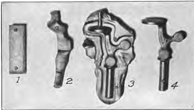
Fig. 171. Steps in Forging Automobile Part
